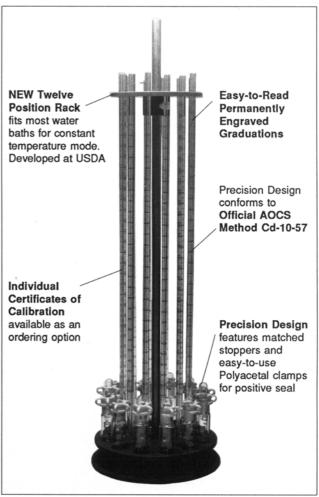
Dilatometer for the determination of the solid fat index (an empirical measure of the solid fat content) of shortenings, margarine oils, and other fats with a solid index of 50 or less at 10°C. Results are expressed as melting dilation in mL/kg of fat.
